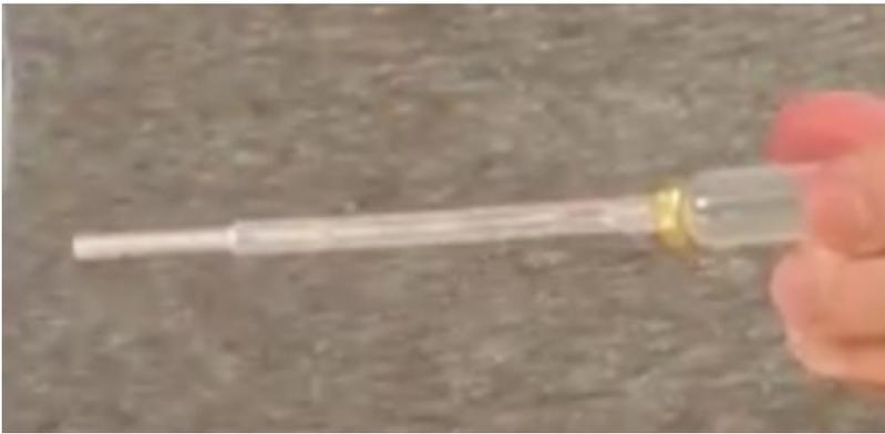
1. Screw a hex nut onto two plastic pipettes
