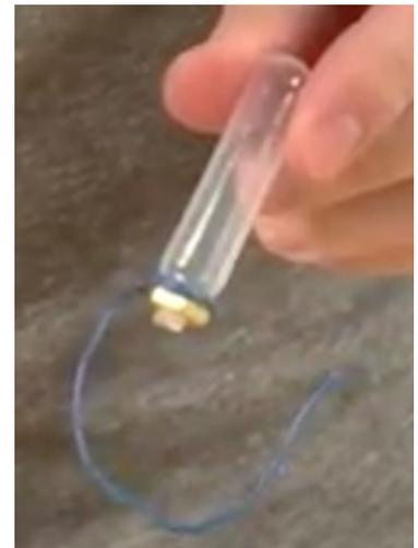
4. Fill up the 'loop' pipette bulb with just enough water so it barely sinks. Fill up the 'hook' pipette bulb so it barely floats.
